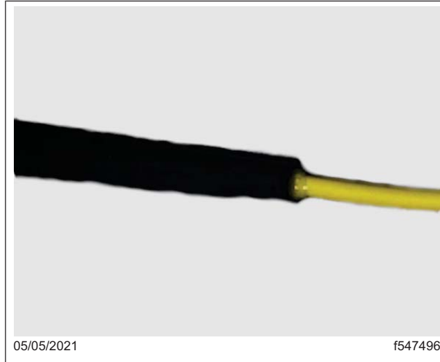
Fig. 21, Tube Sleeve with Adhesive
