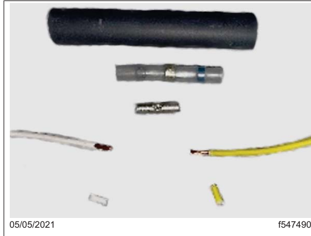
05/05/2021 f547490 Fig. 15, Tube Sleeve, Solder Sleeve, Barrel Connector, and Prepared Wires
