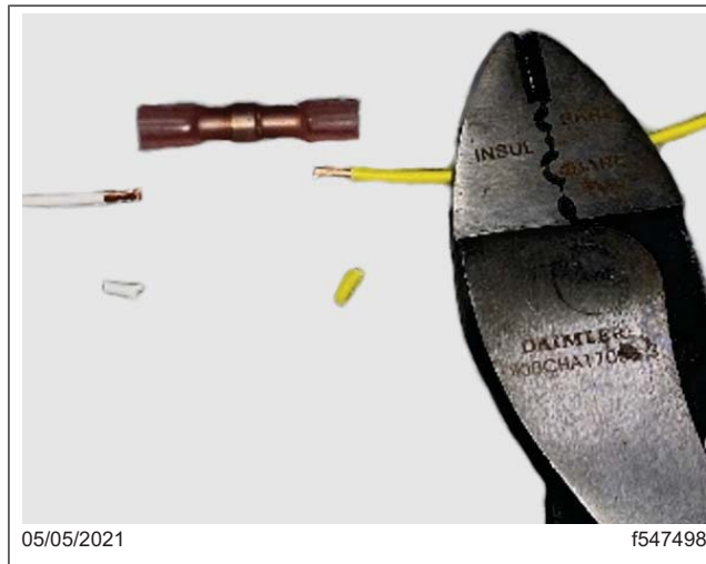
Fig. 22, Sta-DRY Connector, Prepared Wires, and Crimping Tool
