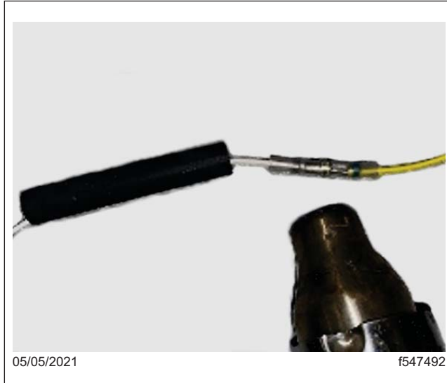
Fig. 17, Heating the Solder Sleeve
