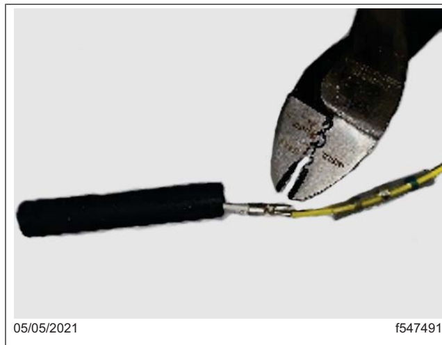
05/05/2021 f547491 Fig. 16, Crimping With DK10CHA17003-3 or Similar Tool
