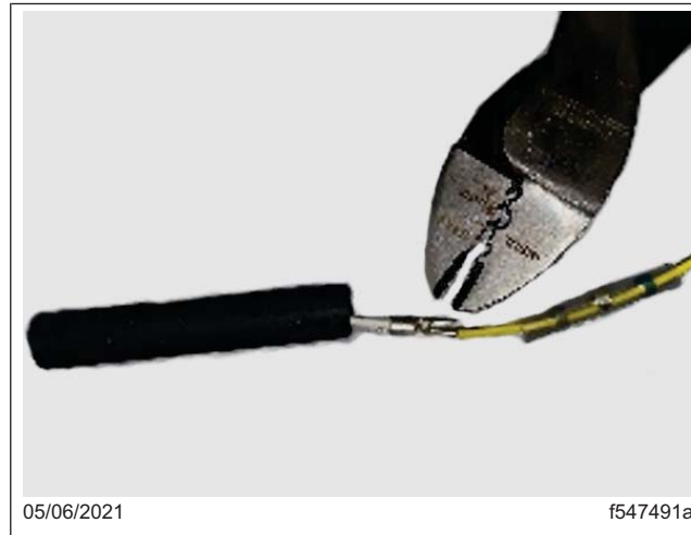
Fig. 23, Crimping With DK10CHA17003-3 or a Similar Tool
