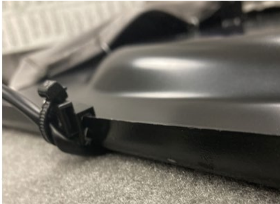
Fig. 5, Proper Clipping and Routing of Harness Driver Seat Sensor
