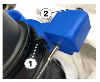
5. The oil filter housing has two small injection molding seams on either side. The tool will align with the seams and lock into place (1).
