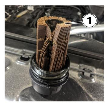
For example, the filter paper is torn, and the lower plastic section remains stuck inside the engine oil filter housing (1).
