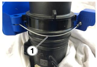
4. Ensure the cable is positioned correctly on the side of the oil filter housing (1).
