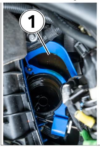
13. After reinstalling the new oil filter and oil filter, torque the oil filter cap to a repair instruction specification.
