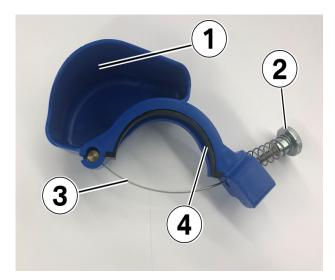
1. Install special tool 83 30 5 A3B 354 BMW Oil Catch onto the side of the oil filter housing.
