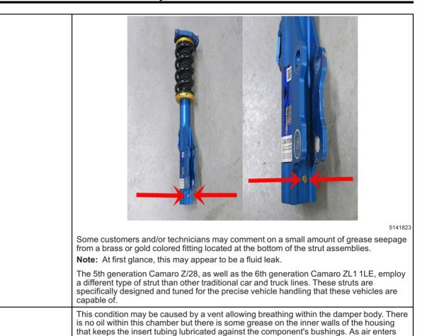
and exits this vent, it is normal to have small amounts of this grease exit the strut. This is
