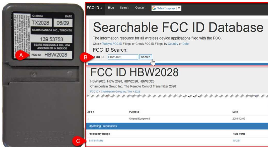
Figure 1. Checking the operating frequency.
