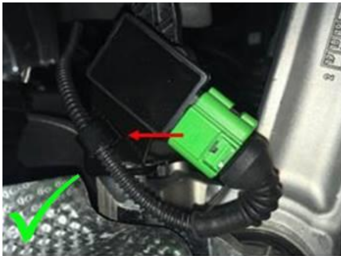
Figure 3. Correct positioning of the harness clip. The clip is mounted on the sensor side of the bracket.
