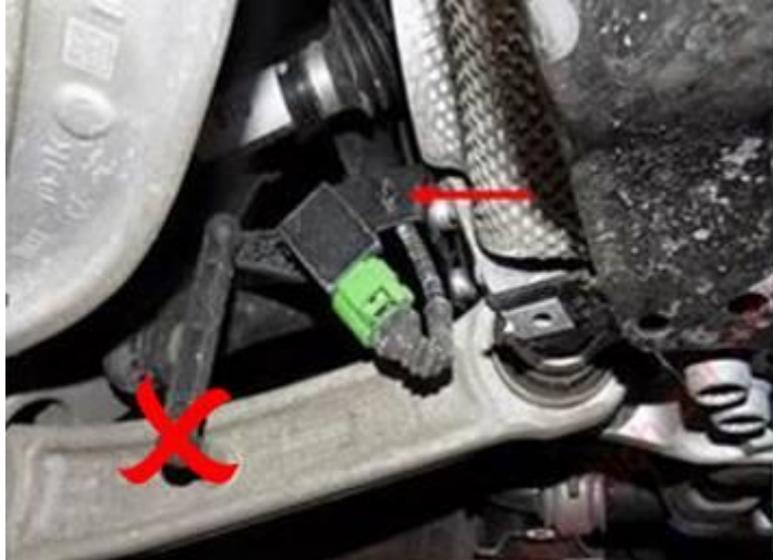
Figure 2. Incorrect position of the harness clip. The clip is mounted on the opposite side of the sensor bracket.
