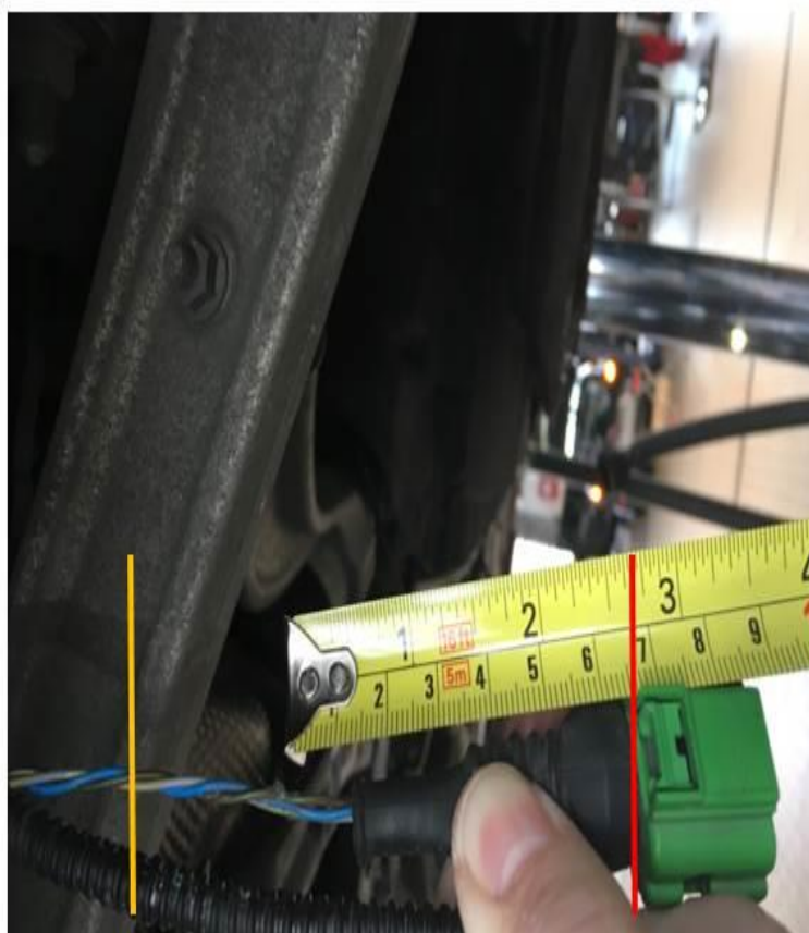
Figure 1. The affected area located under the corrugated tube between the red and yellow mark.
