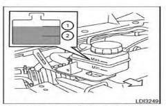
Check the fluid level in the reservoir. If the fluid is below the MIN line(2) or the brake warning light comes on, add Genuine NISSAN brake fluid CLARIANT 6M DOT4 or equivalent DOT4 up to the MAX line(1). If the fluid must be added frequently, the system should be checked by a NISSAN dealer.
