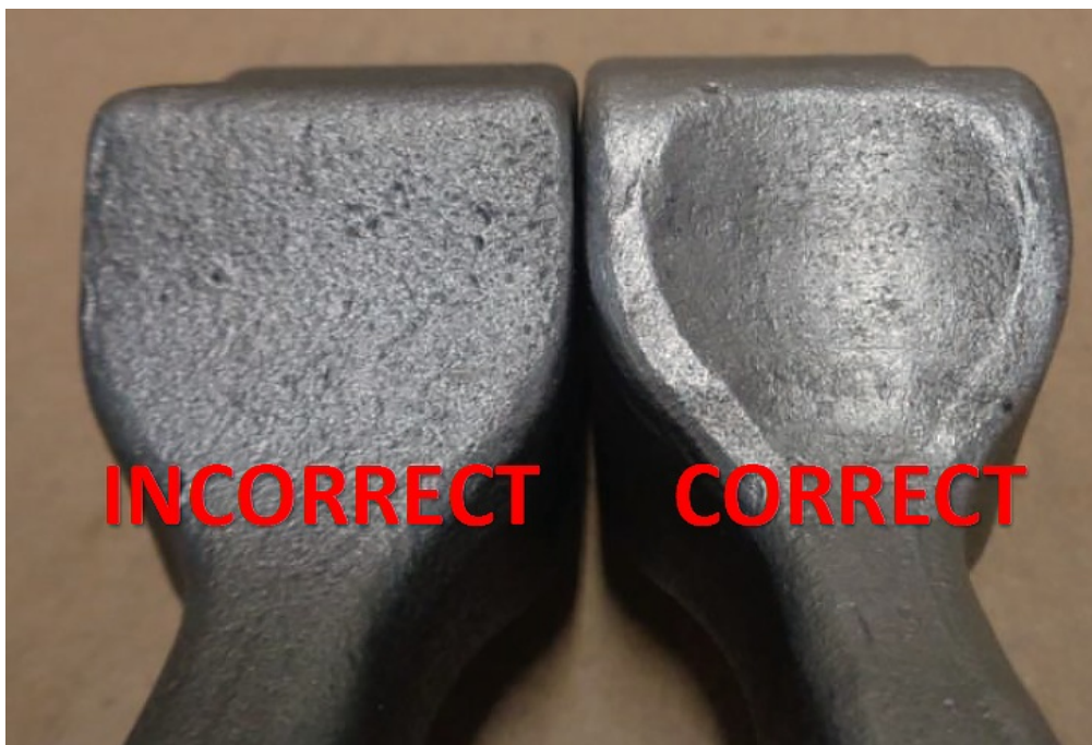
INCORRECT LOCKING MECHANISM. INTERNAL LOCK IS STRAIGHT.
