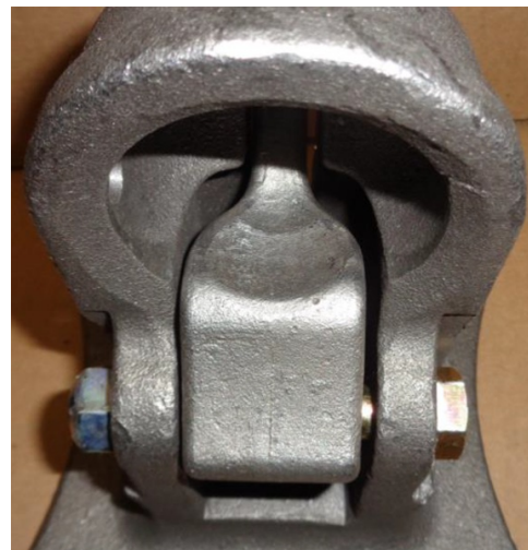
CORRECT LOCKING MECHANISM. INTERNAL LOCK HAS A RADIUS
