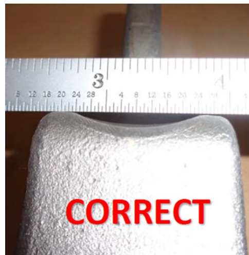
CORRECT LOCKING MECHANISM. INTERNAL LOCK HAS A RADIUS
