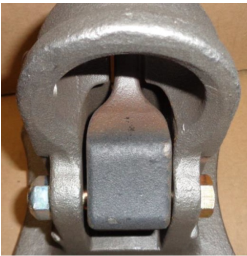
INCORRECT LOCKING MECHANISM. INTERNAL LOCK IS STRAIGHT.
