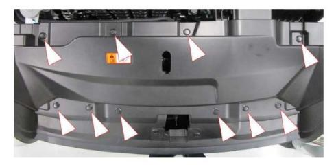
2. Remove the Latch Cover (secured with 2 bolts):
