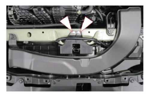
3. Loosen 2 bolts which secure the Latch to the Body and move Latch down to its lowest position.
