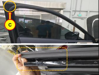
2. Attach the glass run pad (D) as shown in the photos.
