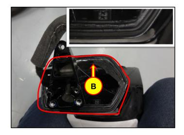
3. Attach the pad to the side view mirror seal.
