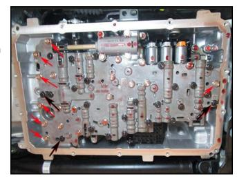
9. Remove 9 bolts and remove the E-module.
