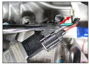
11. Remove 2 mounting bolts and remove the position sensor.
