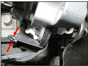
10. Push down on the tab on the position sensor connector and push the lock tab in the direction shown.
