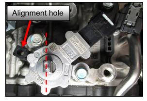
13. Install the correct alignment tool in the hole on the transmission and the alignment hole on the position sensor. Tighten both bolts that secure the position sensor.
