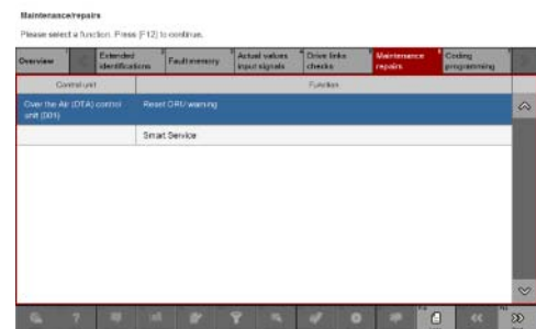
Resetting ORU warning
