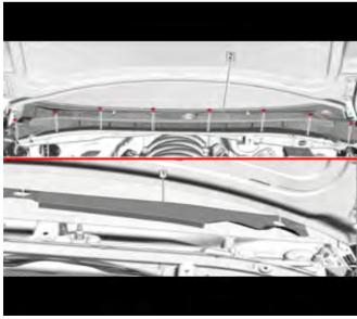
**Note:** Prior to installing the air inlet grille panel, again verify there is 20 mm (0.80 in) minimum clearance to the wiper arm cycle.
