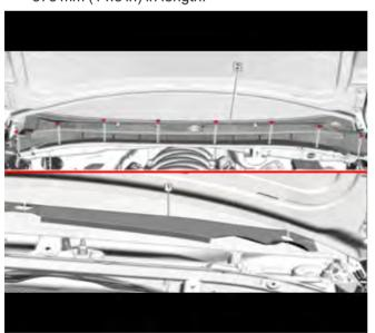
Remove the air inlet grille panel (2) and the windshield wiper system module shield (1). Refer to Windshield Wiper System Module Shield Replacement in SI.
