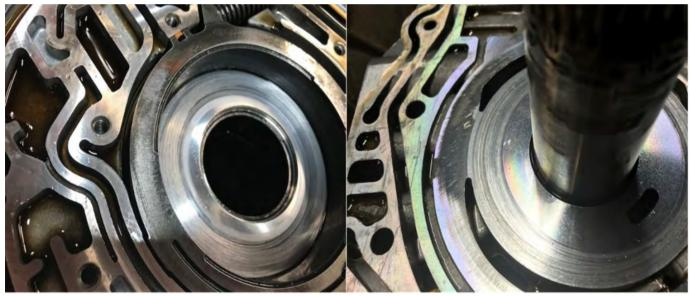
**Note:** Refer to the latest version of PI1447 for possible bushing/shaft scoring. Replace parts as necessary.
