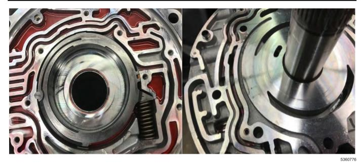
**Do Not** replace the pump if no signs of damage or excessive wear was not validated during inspection as shown above.
