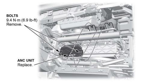
3. Install the parts in the reverse order of removal.
