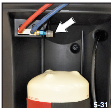
Contaminated Refrigerant Recovery Machine Connection Port
