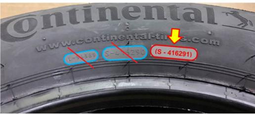
**VERY IMPORTANT:** When performing these inspections, <u>BOTH</u> the DOT Serial Number and the Mold Number (circled in **RED**, **Highlighted and In Parentheses**) must match those provided in the photos above. If only one of the 2 numbers match, the tire(s) is not affected.
