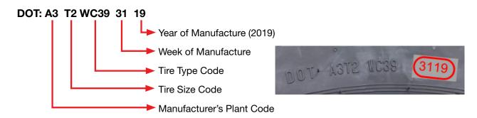
2. Mold number is located on the sidewall of each tire.
