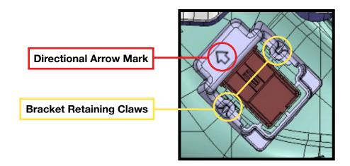
STEP 3) Install the bracket by pushing it on to the door panel while aligning the retaining claws. Ensure the fitment and retention strength is sufficient. CAREFULLY reinstall all parts in reverse order and perform a function test of the seat memory switch. Reset the seat memory positions (and PRG memory height) gate to match the customer's previous selections.
