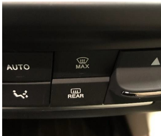
Figure 1: Defrost button of the A/C Control Panel stuck in pressed position.
