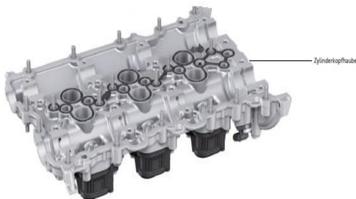
Figure 4. Remove the cylinder head cover and gasket.
