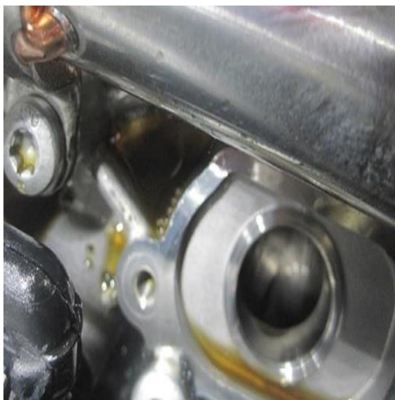
Figure 2. Oil in the Audi valve lift system.
