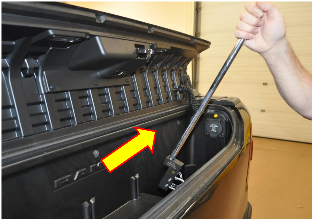
Bending the striker upwards to raise lid.
