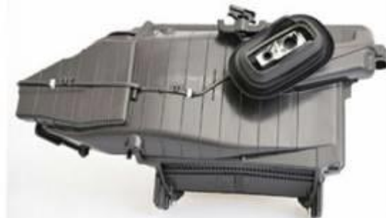
Figure 1. HVAC evaporator and housing.
