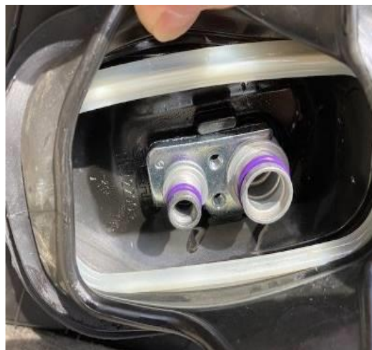
Figure 3. Refrigerant connections to the expansion valve.
