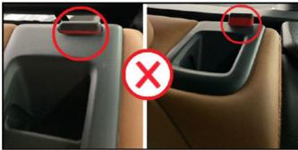
Check rear seat backrest lock operation and rework release cable (if necessary).
