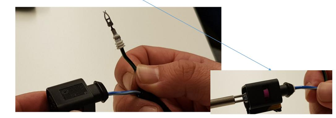
Before plugging adjust the terminal wing by slightly pull it up. This to be able to keep the retention force of the terminal OBS! If wing will be broken terminal need to be exchanged.
