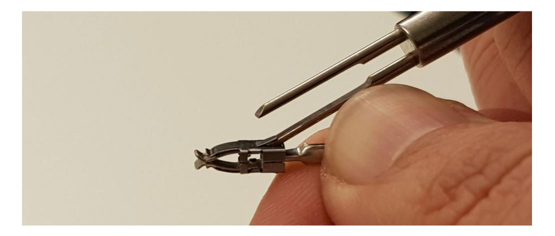
Currently cavity 1 is having BU/WH cable. This one shall be pushed in to cavity 2. BK/GN which is in cavity 2 shall be added in to cavity 1
