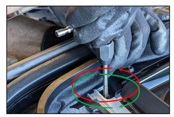
3. <u>Apply blue liquid thread locker</u> and tighten the retaining bolt (A) to specifications.
