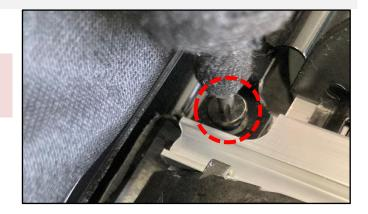
2. Inspect the receiving threads for damage and use a tap bit (M5 \*0.8P) and <u>carefully align</u> to repair threads.
