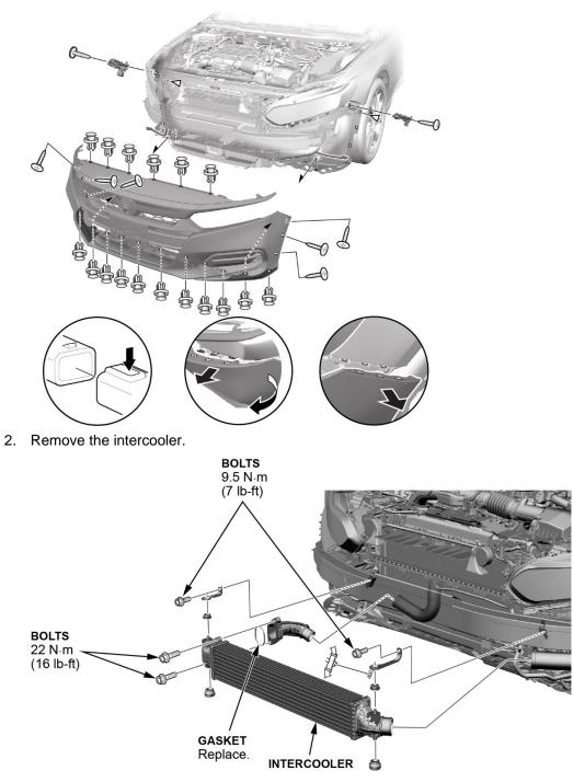
3. Install the new intercooler and gasket, and torque the two bolts mounting the intercooler to 22 N·m (16 lb-ft) and the two bolts with brackets to 9.5 N·m (7 lb-ft).
