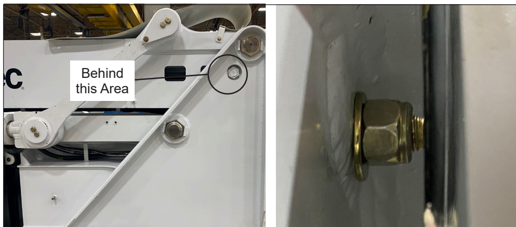
Figure 2 — Elbow Inspection for Hex Nut
