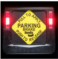
Dash Electronic Control Unit (DECU) Included with the Bendix® Intellipark® EPB System
