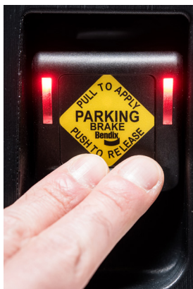
PUSH the switch to release the parking brakes.
