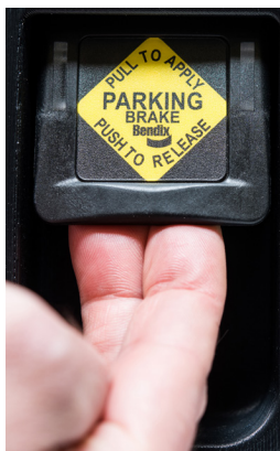
PULL the switch to engage the parking brakes.
