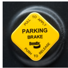
Pneumatic Push/Pull Knobs Replaced by the Bendix® Intellipark® DECU (Switch)
