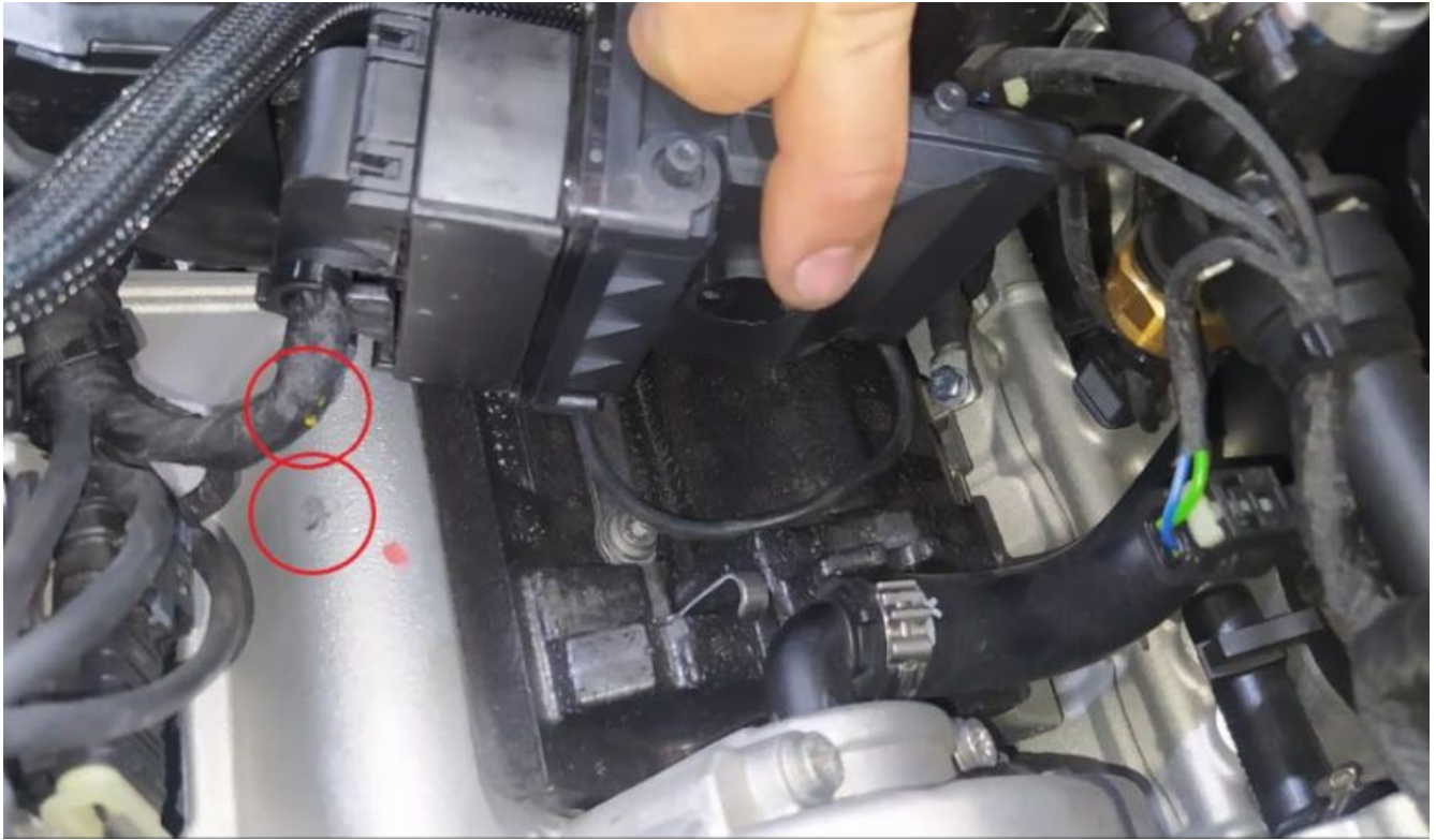
Figure 2: CHAFING MARK ON THE WIRING HARNESS AGAINST THE CRANKCASE
