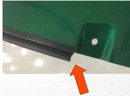
Figure #1 - Trim Lok Seal Installed
