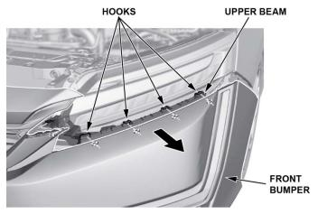
9. With the help of an assistant, remove the front bumper and undercover as an assembly. Disconnect the connectors. **CONNECTORS**
