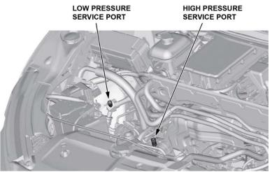
2. Evacuate the A/C system. Measure the amount of refrigerant oil removed from the A/C system after the recovery process is completed.
