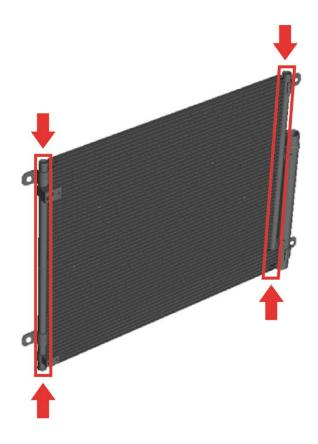
18. Check the inlet and outlet joints and the receiver/dryer cap for leaks.
