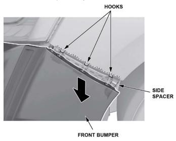
8. Remove the front bumper from the hooks on the upper beam.
