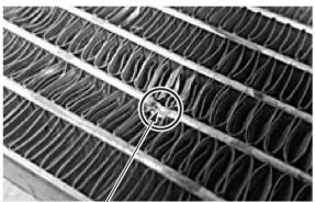
Impact damage on the tube face.
