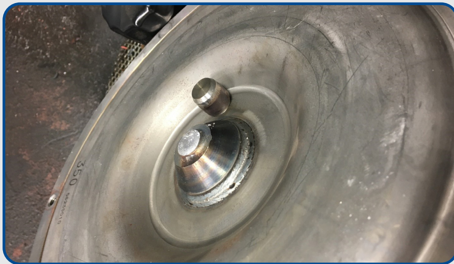
Torque converter with broken nose.
