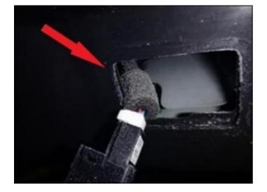
1. Start wrapping from the middle of the switch and continue upwards until the thick rubber foam and the border between it and the harness are completely covered.
