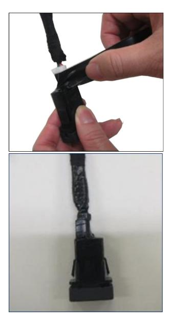
2. After reaching the border between the thick rubber foam and the harness, cut the tape once. Then, start wrapping again in the reverse direction (i.e. start from where the tape was cut and stop at the middle of the switch). After cutting the tape once more, wrap upwards again to ensure no gaps are left.
