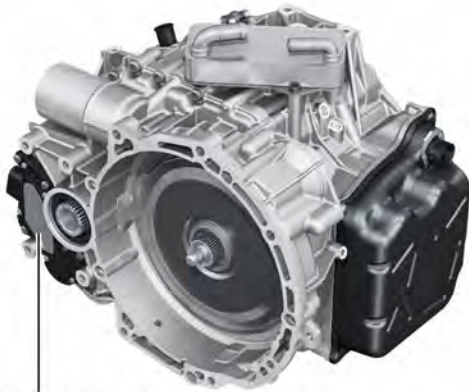
Auxiliary hydraulic pump 1 for gearbox oil V475
