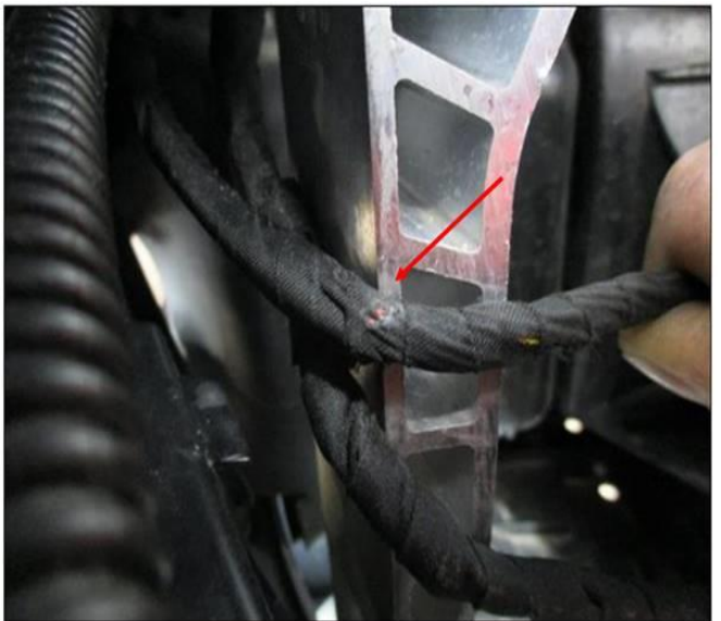
Figure 2. Example of parking aid harness that has chafing.
