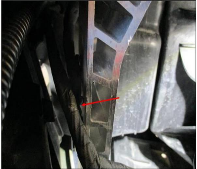
Figure 1. Example of parking aid harness that has chafing.
