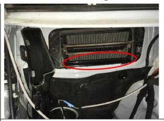
A mirror is helpful for checking the lower area of the sealing frame.
