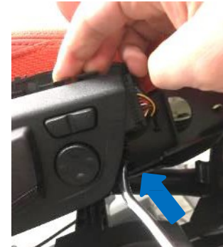
3.3 Disassembly the rear side
