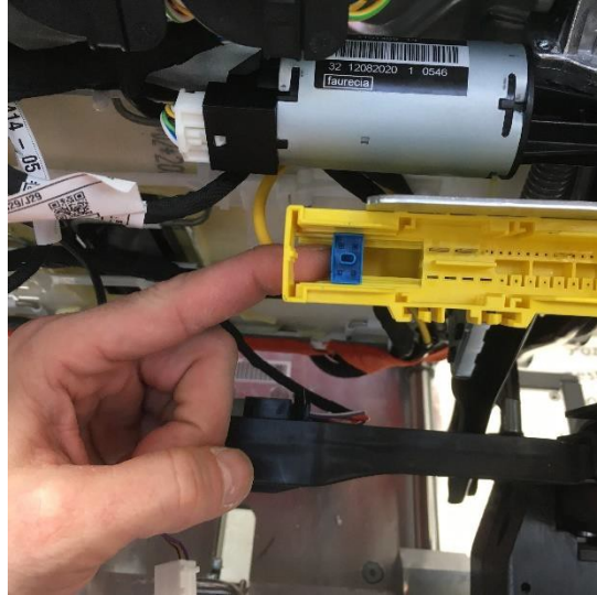
10.2 Mount the airbag plug to the central plug
