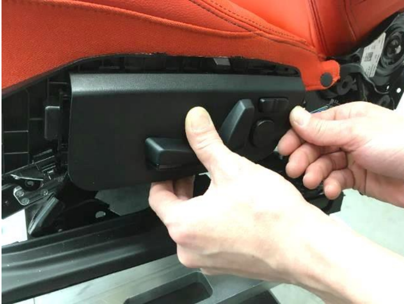
13.1 Assembly the adjuster on all clips – correct assembly -> click noise
