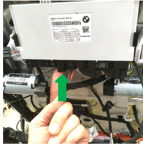
8.2 Connect SHG cushion plug to the memory unit
