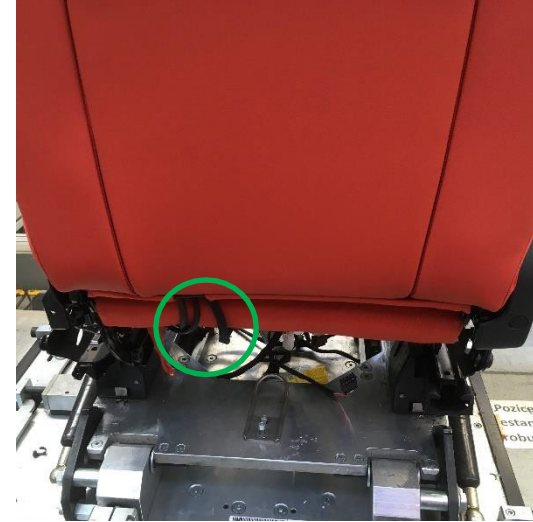
4.3 The cables must be routed through the hole in the cover
