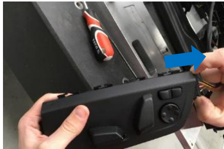
3.5 Press and remove cable connector
