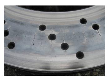
1. Visible cracks are caused by high thermal stresses during rapid heating and cooling of the brake discs. Braking from high speed with cold brake components (less than 212 degrees F) increases the likelihood of cracks to form. These hairline surface cracks are usually spread over the entire brake disc friction area, and have no negative influence on the durability or braking performance.
