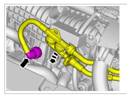
Undo the hose from the connection. Fold marked part aside.
