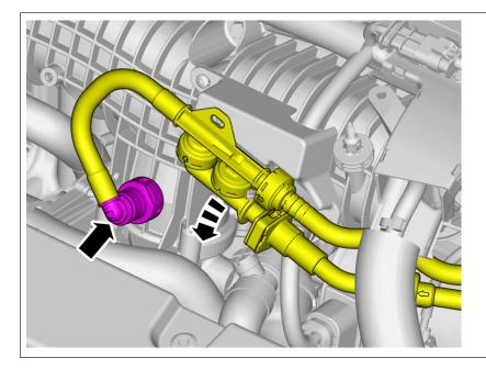
Undo the hose from the connection. Fold marked part aside.
