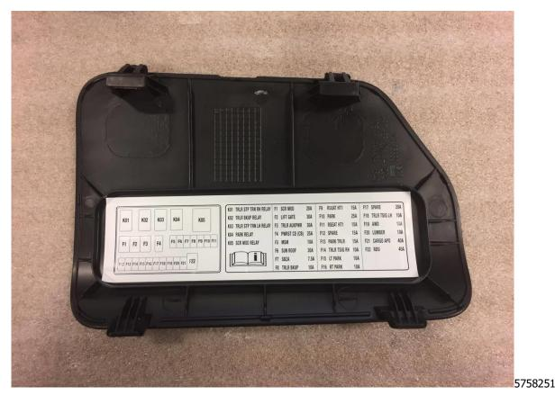
3. Install the new fuse block label as shown above.
