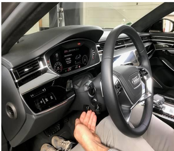
Figure 1. 40 kg force pushing steering wheel upward.
