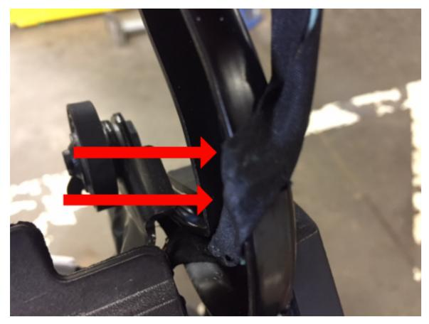
If any harness damage is found, repair as necessary.
