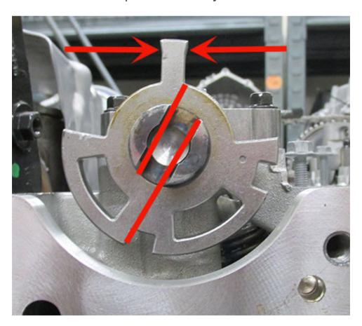
Photo below is showing the proper relationship between the 2D matrix marking and the small tang on exhaust cam reluctor wheel.
