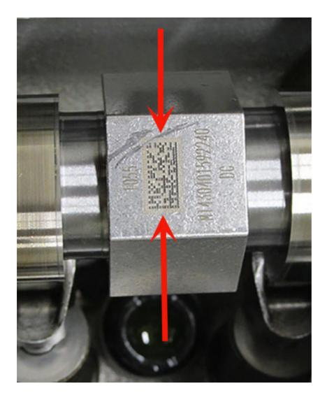
Once the exhaust camshaft 2D matrix has been positioned at 12' O'clock. Verify the small tang located on the camshaft reluctor ring (Arrows below showing tang on reluctor) is inline with the 2D matrix marking. Also shown are additional reference points used to verify exhaust cam reluctor orientation to camshaft.
