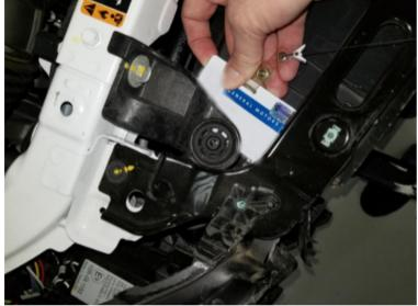
If this is the cause of the sound or vibration, it can be verified in the stall by evaluating vehicle idle noise/vibration and/or raising the engine RPM in Drive to 1200-1300 with foot on brake. While at this engine speed, have a helper remove the bolts on the radiator upper brackets. The noise or vibration should improve or go away. If it does, retighten the bolts to 14 Nm (10 lb ft) and tell the customer Engineering is working on a fix for this.
