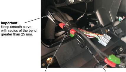
Attach couplers to the main span with tape to prevent any rattles (roughly in line with existing PVC tape on the tube). Attach the MOST cord at the same location.
