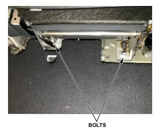
16. Remove the third row lower seat cushion by removing the three bolts.
