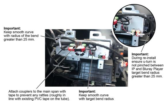
28. Install all of the removed parts in the reverse order. When installing units, make sure the harness is routed correctly. A mis-routed harness can put pressure on the wires and connectors causing connection issues. Do not pull on the units or MOST feeders while the FAKRA connectors are connected to help prevent communication issues.
