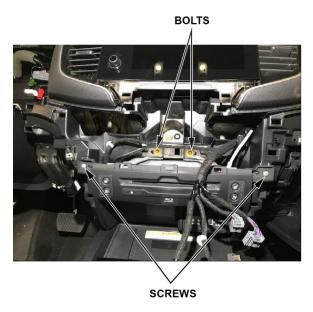
12. Loosen the two bolts holding the infotainment unit, then remove the unit.
