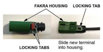
21. Repeat steps 17 thru 20 for the other connectors. Then, install the FAKRA connectors to the infotainment unit and tuner unit.
