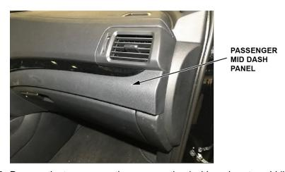
10. Remove the two screws, then remove the dashboard center middle trim.
