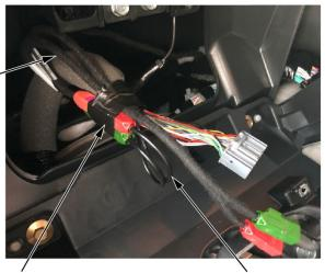
Attach couplers to the main span with tape to prevent any rattles (roughly in line with existing PVC tape on the tube). Attach the MOST cord at the same location.
