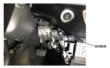
5. Pull back the dash panel to allow the meter bezel removal.
