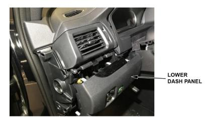
4. Remove the screw to loosen the dash panel.
