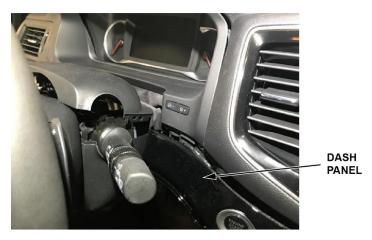
6. Disengage the clips around the meter bezel, then remove the bezel and upper column cover as one piece.
