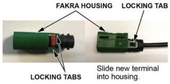
25. Repeat steps 21 thru 24 for the other connectors. Then, connect the FAKRA connector to the infotainment unit and tuner unit.
