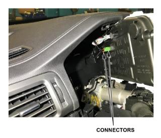
8. Remove the hazard switch panel.
