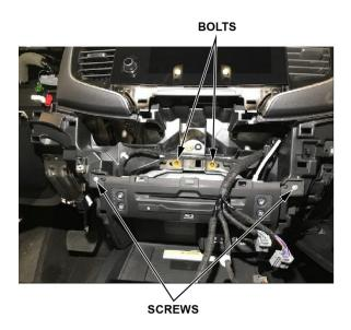
12. Loosen the two bolts holding the infotainment unit, then remove the unit.
