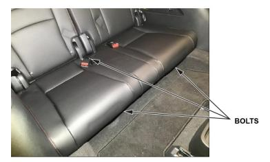
17. Remove the two front bolts for the passenger third row seat-back.
