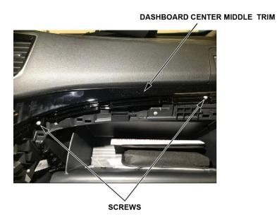
11. Remove the two screws and bolts, then remove the dashboard center lower panel or accessory CD player.
