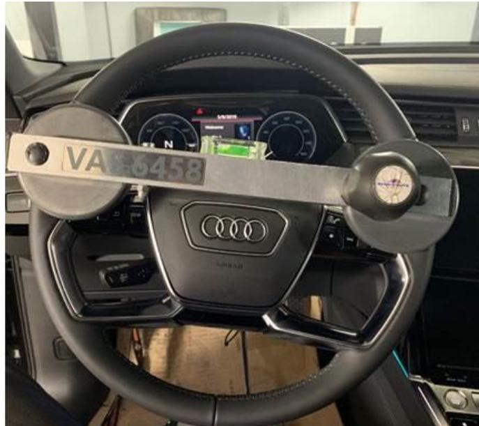
**Figure 1.** VAS 6458 installed with steering wheel off-center.
