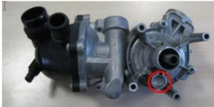
Figure 2. Coolant marks in the plug of the coolant pump housing.
