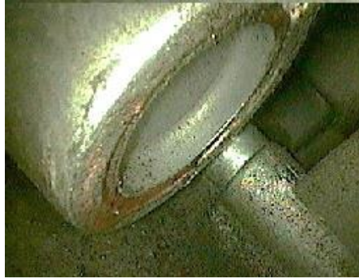
Figure 3. Coolant marks on the flange of the coolant pump housing.
