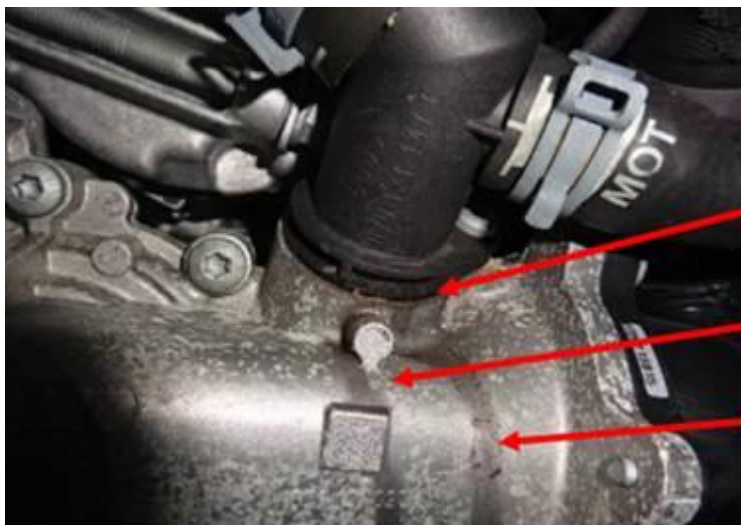
Figure 6. Areas where coolant marks can be found.
