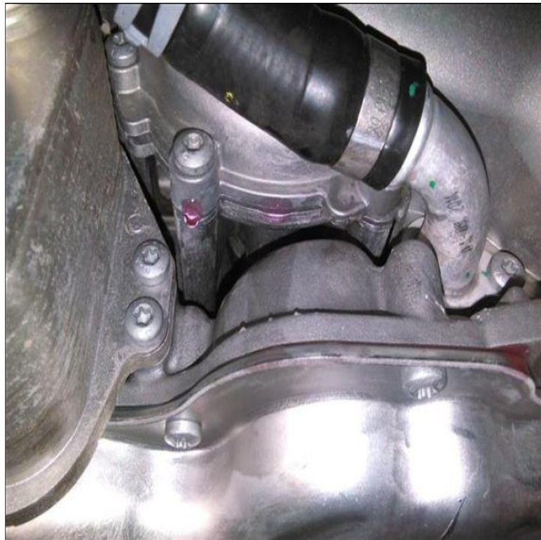
Figure 4. Coolant marks on the flange of the thermostat housing.
