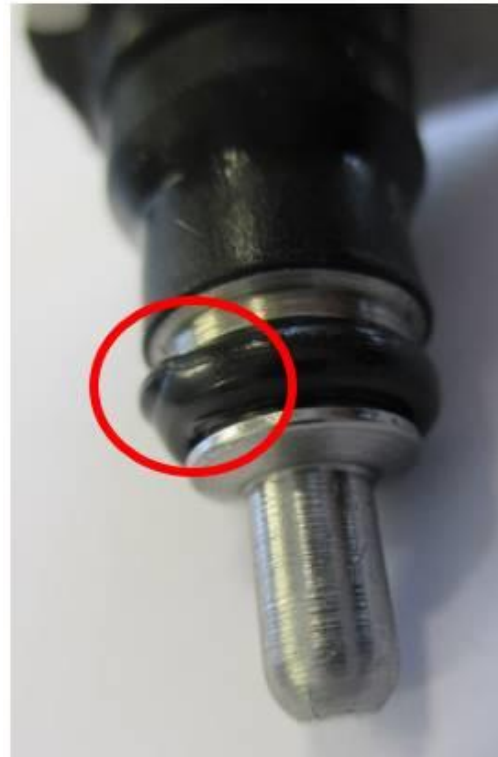
Figure 1. O-ring is pinched.
