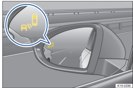
Fig. 2 In the outside mirror: Visual indicators for Side Assist.
